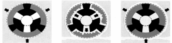
Figure 2: Action of neoprene 'one-way' valves
